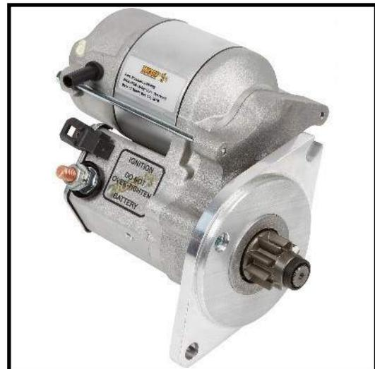
Whether there is one wire running to the starter from the solenoid as on early MGs or three as on later cars, the gear reduction starters can be configured to work.
