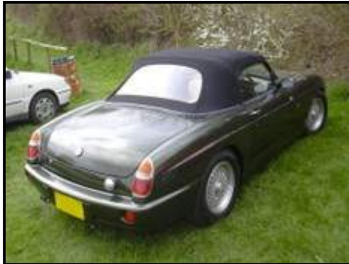
Although it looks like an MGB, the only panels shared with the original are the doors and trunk. The body-in-white was a reproduction made by British Motor Heritage (who started making MGB bodies in 1988), modified with the wider fenders made by Abbey Panel on the RV8 to accommodate wider rubber at all four corners.
